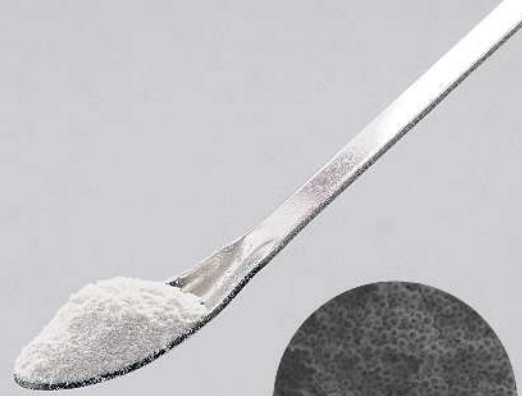
Morphology of AKSOPEEK powder particles
